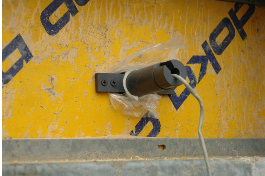
Figure 3 —Bracket with Pressure Transducer Attached to Formwork
