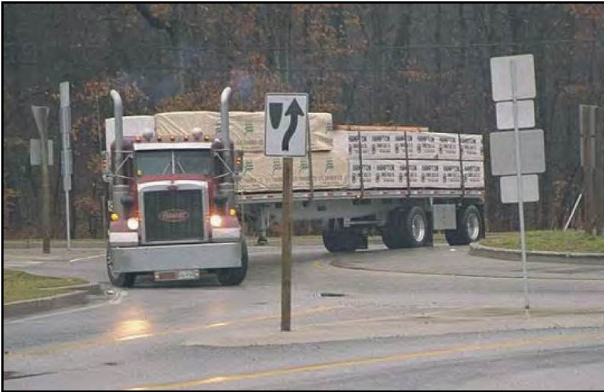
LARGE TRUCK OVERTOPPING THE TRUCK APRON
