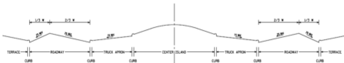
CIRCULATORY ROADWAY AND TRUCK APRON CROSS SECTION
