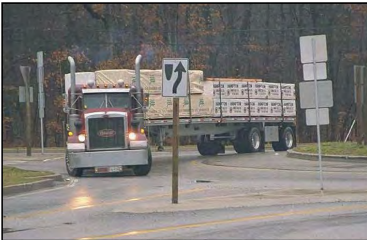
LARGE TRUCK OVERTOPPING THE TRUCK APRON
