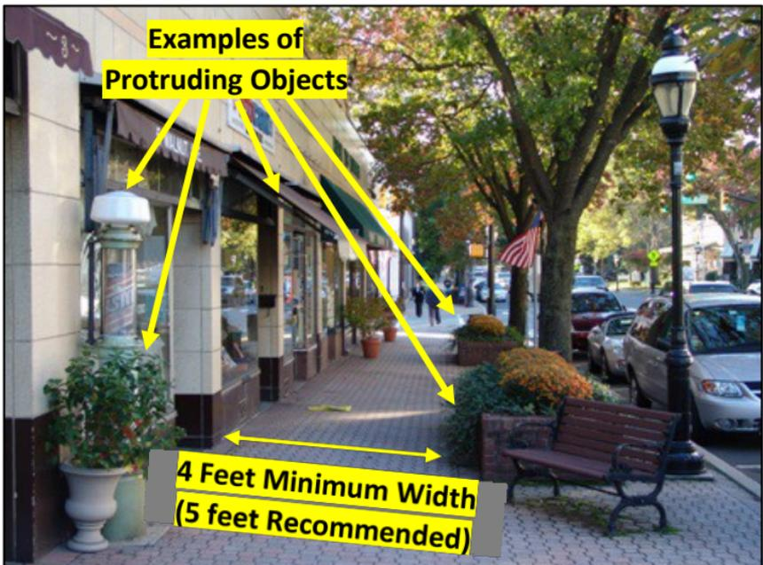
Figure 21: PAR Clear Width Excluding Protruding Objects
