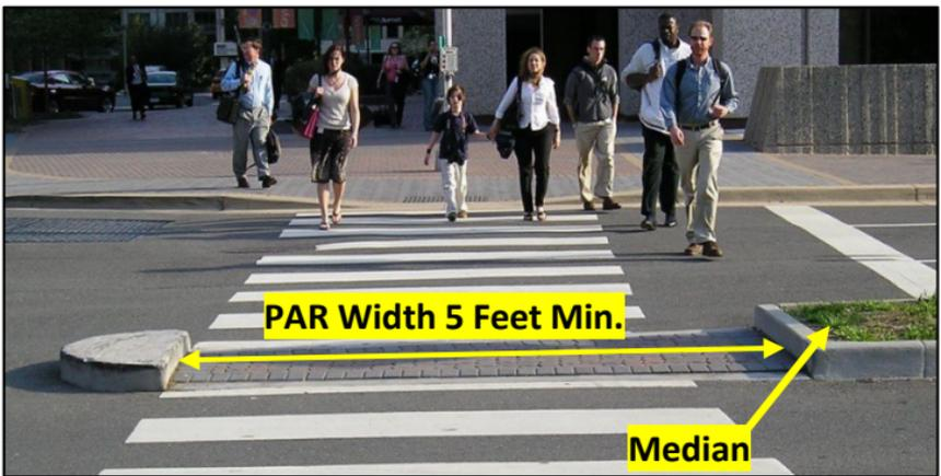
Figure 70: PAR Width within Pedestrian Street Crossings
