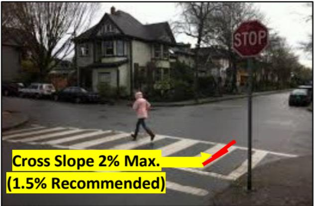
Figure 12: Pedestrian Street Crossing with Stop Control
