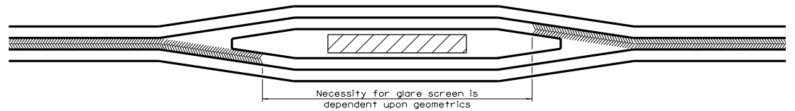
TYPICAL APPLICATION AT MEDIAN OBSTRUCTIONS
