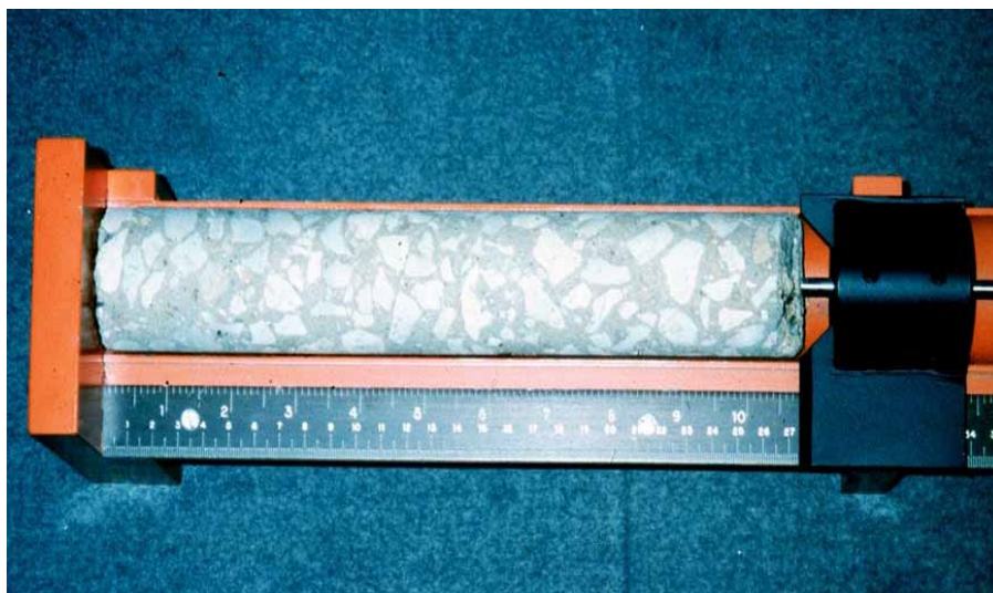
Figure 400-15 — 2-IN. DIAMETER CORE BEING MEASURED IN A CORE MEASURING DEVICE
