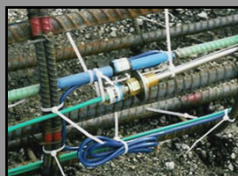
O-cell at base of small shaft to measure end bearing on rock
