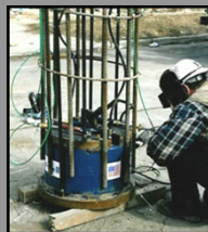
O-cell at base of small shaft to measure end bearing on rock
