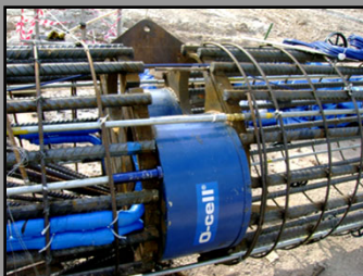
Two O-cells at the mid-level of shaft measuring shaft friction to a total load of 7400 tons
