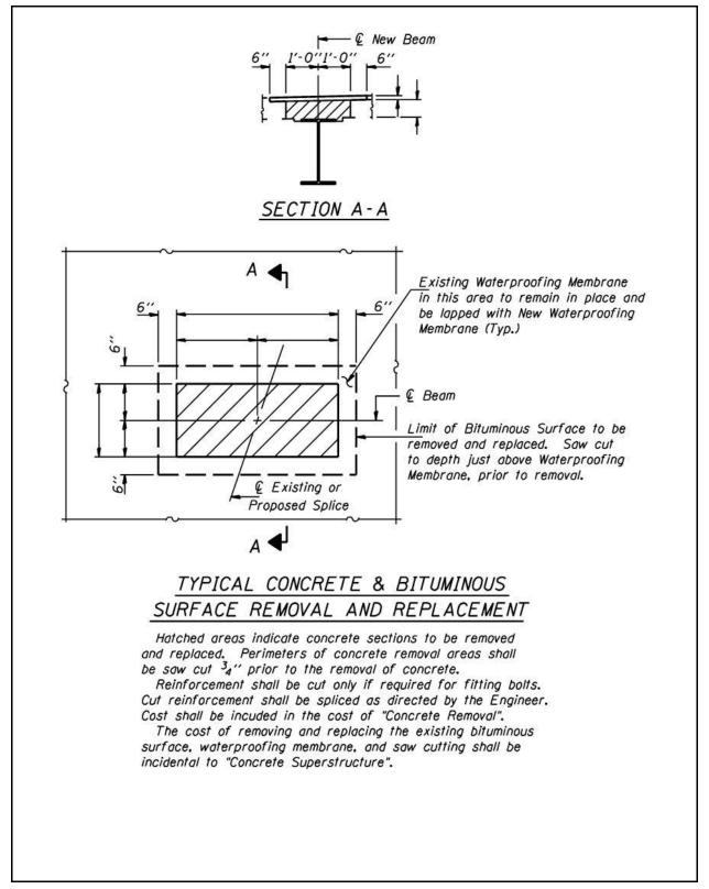
Figure 2.13-8 – Deck Slab Removal for Beam Replacement
