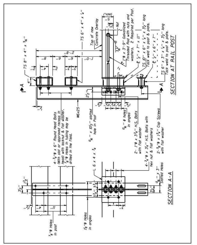
Figure 2.7-2 – Type SM Rail Retrofit on PPC Deck Beams
