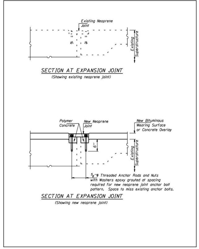
Figure 2.5-21 – Expansion Joint Treatment with Grade Raise and Existing Neoprene
