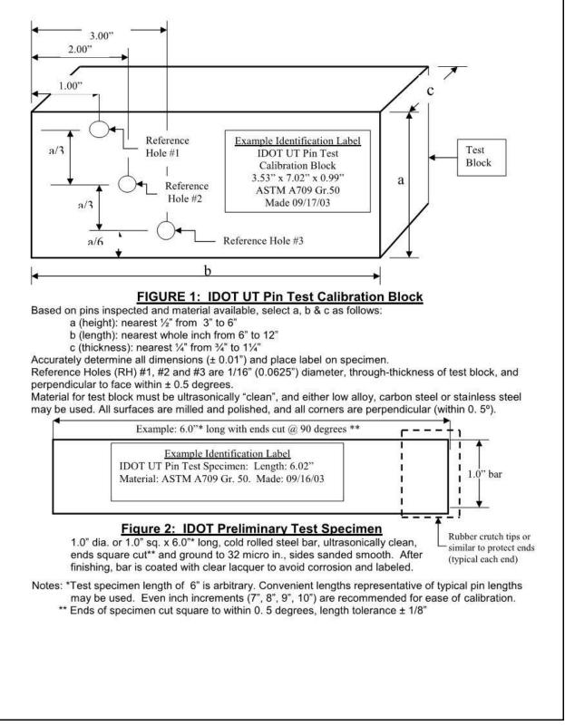
Figure 3.6-1 – Diagram "A" – IDOT Test Block & Specimen
