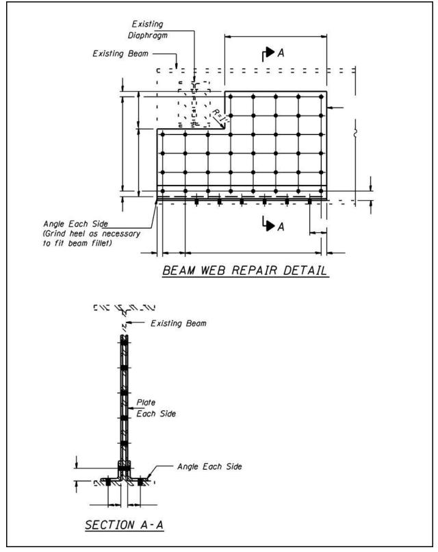
Figure 2.15-3 – End of Beam Repair Detail
