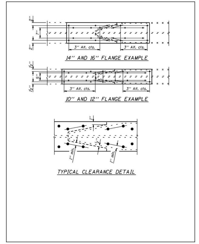
Figure 2.12-3 – Cover Plate Repair Detail
