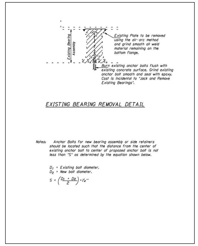
Figure 2.9-1 – Existing Steel Rocker Bearing Removal
