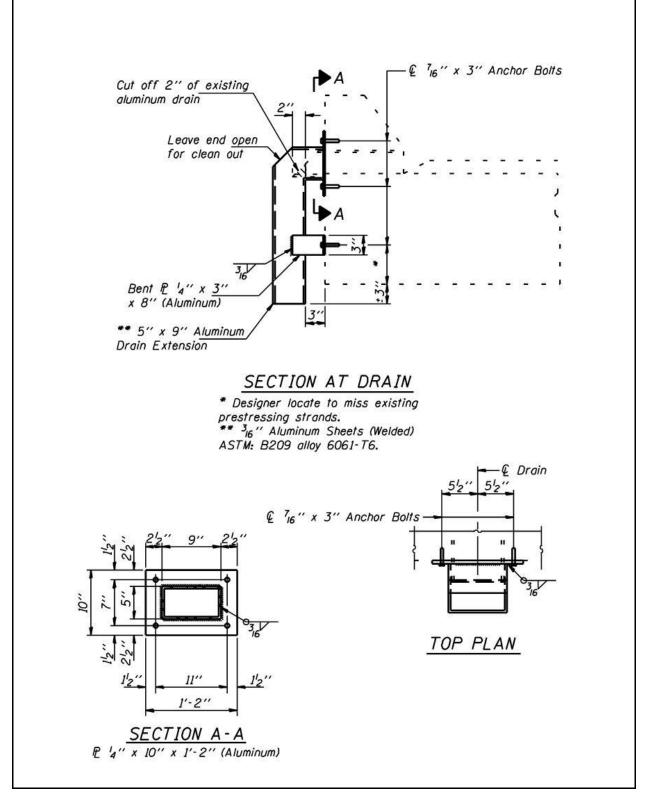
Figure 2.8-4 – Drain Extension Detail
