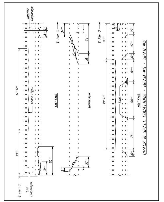
Figure 2.3-7 – Details of Impact Damaged PPC I Beams
