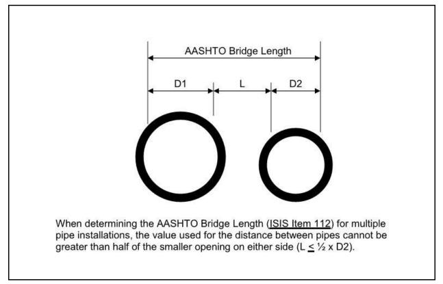
Figure 3.11-1 – Bridge Length for Multi-Pipe Culverts
