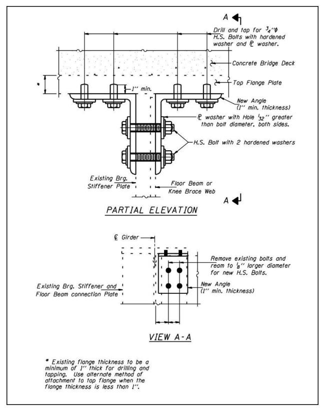
Figure 2.12-6 – Fatigue Repair to Increase Stiffness
