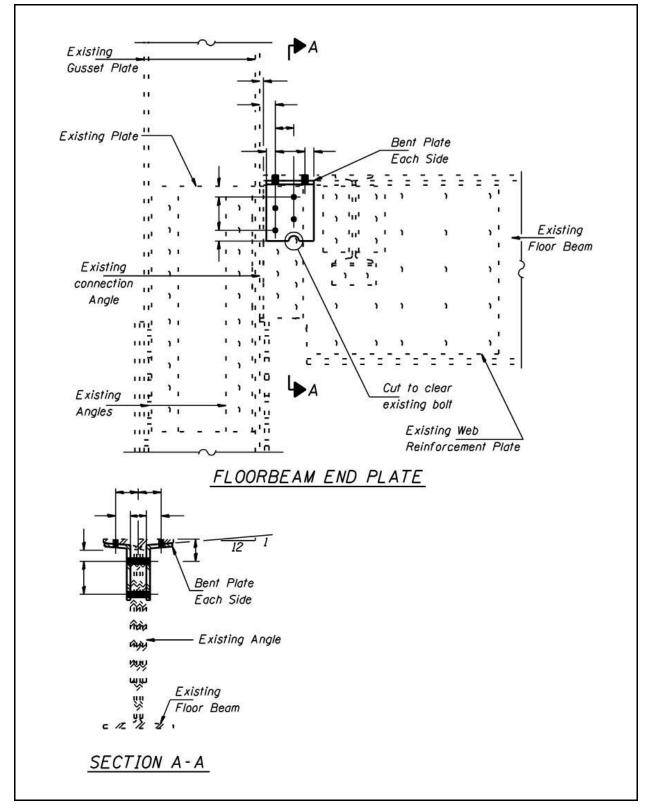
Figure 2.15-11 – Floorbeam Repair
