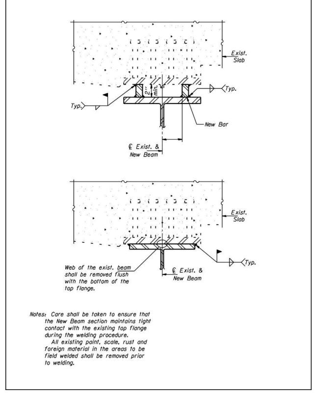
Figure 2.13-12 – Partial Beam Replacement for Composite Beams
