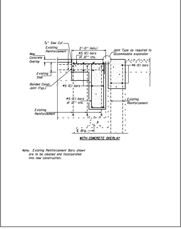
Figure 2.5-10 – R.C. Deck Girder Joint Reconstruction (Full Removal)
