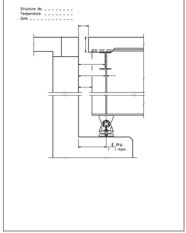
Figure 2.5-18 – Finger Joint Field Dimensions (At Abutment)
