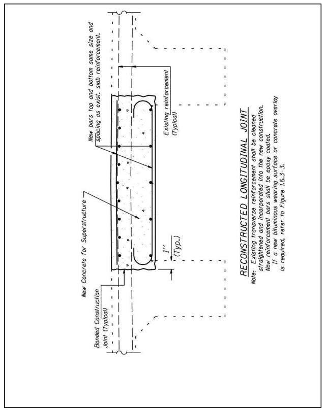
Figure 2.6-5 – Longitudinal Joint Reconstruction with R.C. Deck Girders
