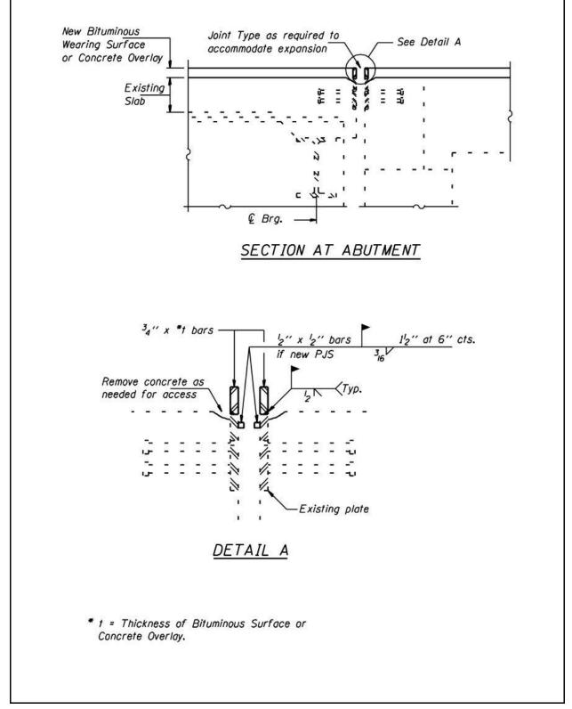
Figure 2.5-5 – Expansion Joint Treatment with Grade Raise and Existing Plates
