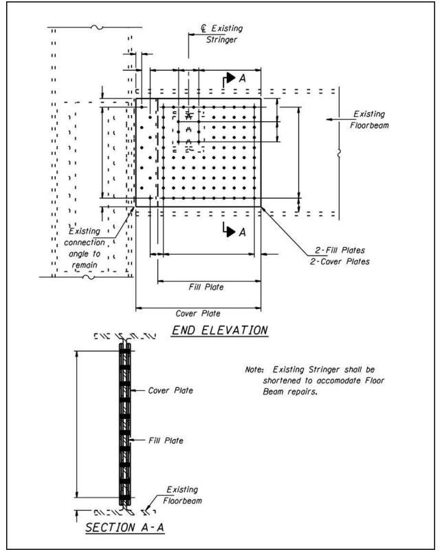
Figure 2.15-10 – Floorbeam Web Repair
