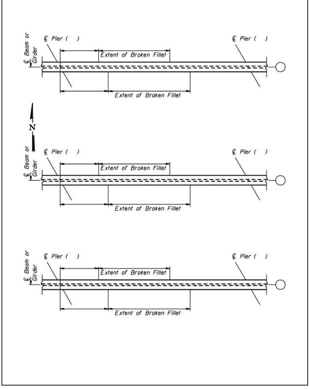
Figure 2.3-5 – Impact Damage Steel Beams Broken Fillets
