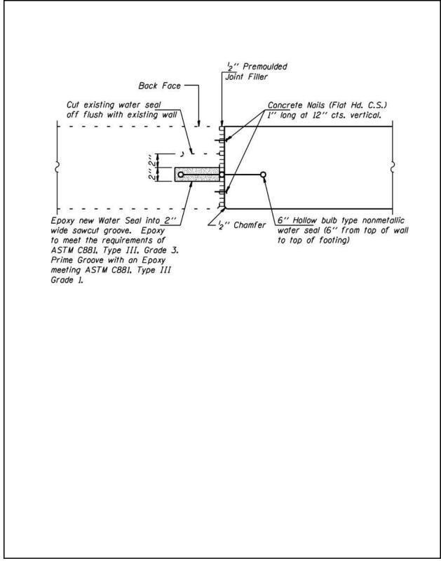
Figure 2.17-5 – Water Seal Replacement Detail
