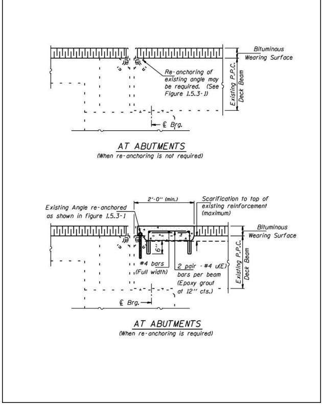
Figure 2.5-14 – PPC Deck Beam Joint Reconstruction
