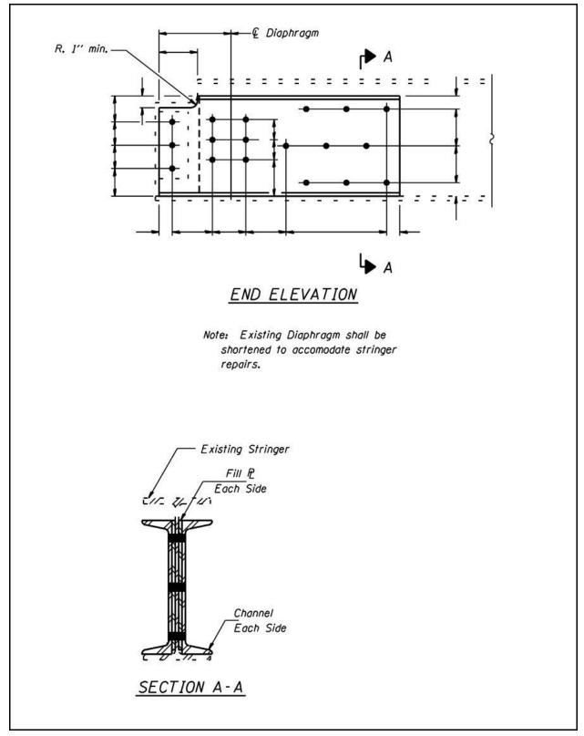
Figure 2.15-6 – End of Stringer Repair Detail
