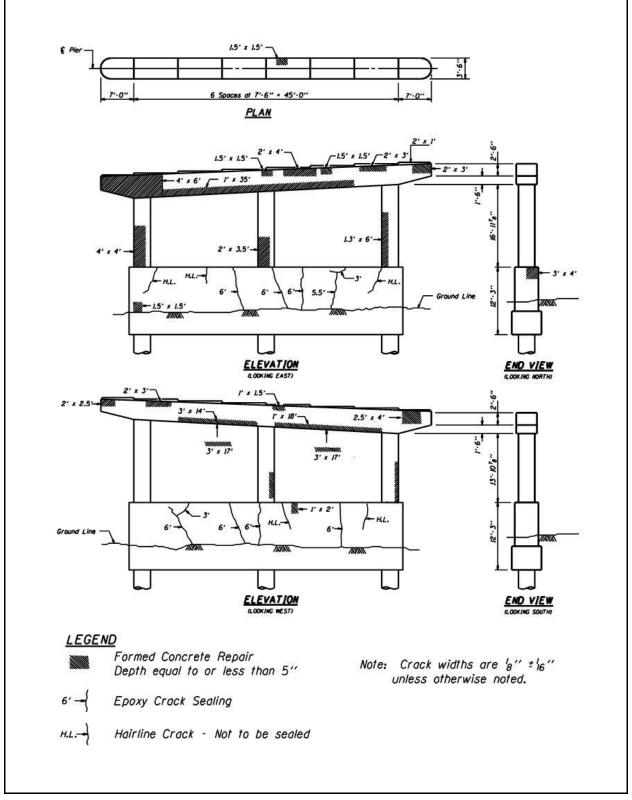
Figure 2.17-1 – Pier Repair Details
