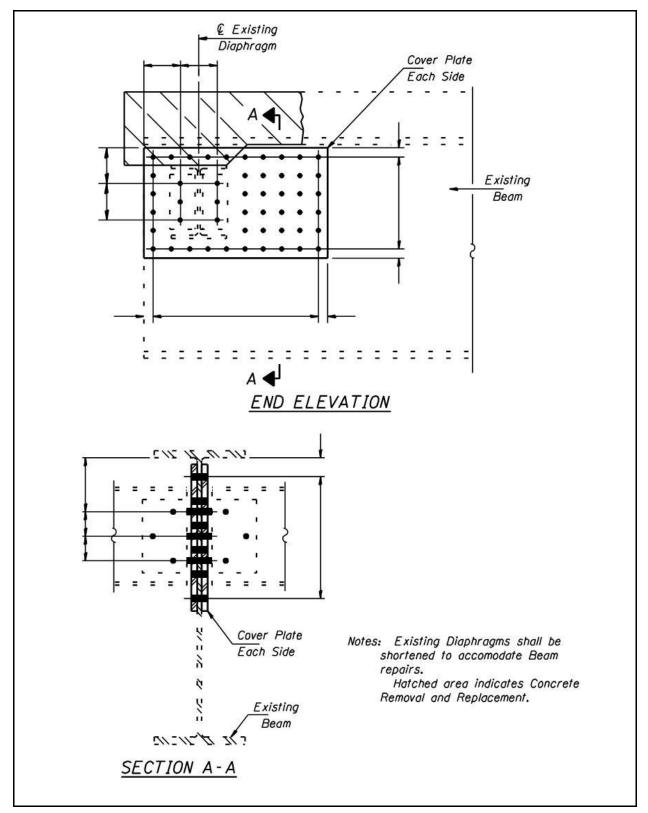
Figure 2.15-1 – End of Beam Repair Detail
