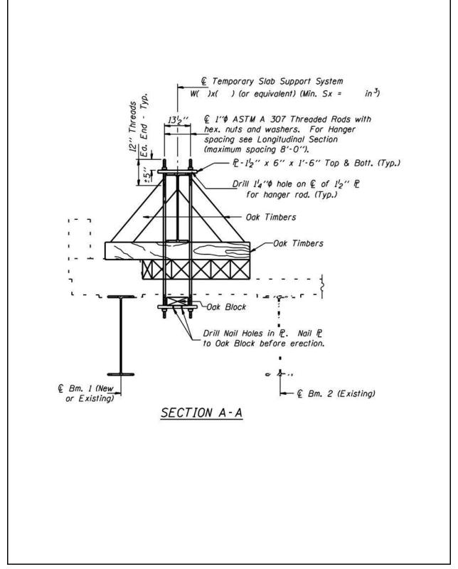
Figure 2.13-10 – Temporary Slab Support Details
