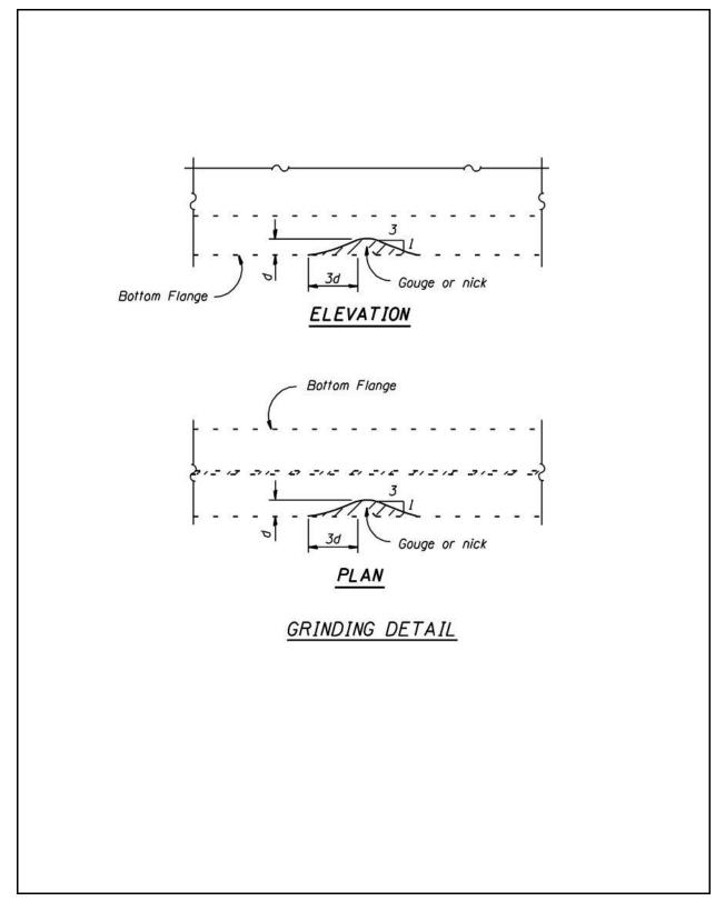
Figure 2.13-7 – Grinding Detail
