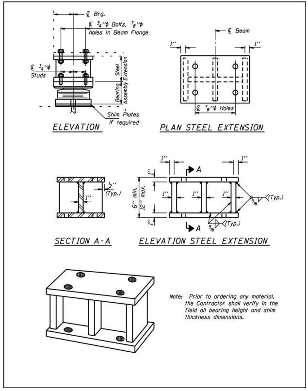
Figure 2.9-3 – Fabricated Steel Extension
