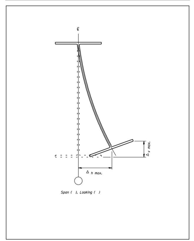
Figure 2.3-6 – Maximum Displacement of Impact Damaged Steel Beam or Girder
