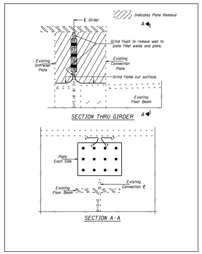
Figure 2.12-4 – Fatigue Repair to Increase Flexibility
