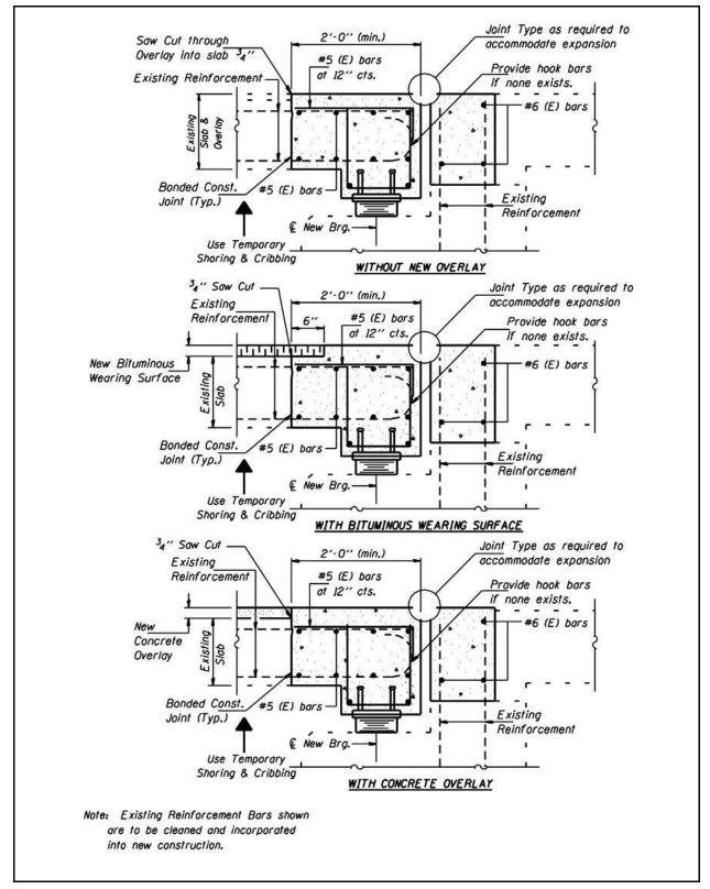
Figure 2.5-11 – Joint Reconstruction for R.C. Slab (Full Removal)
