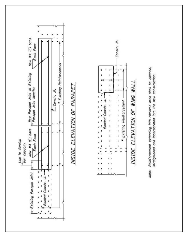
Figure 2.7-7 – Parapet and Wing Wall Repair Details
