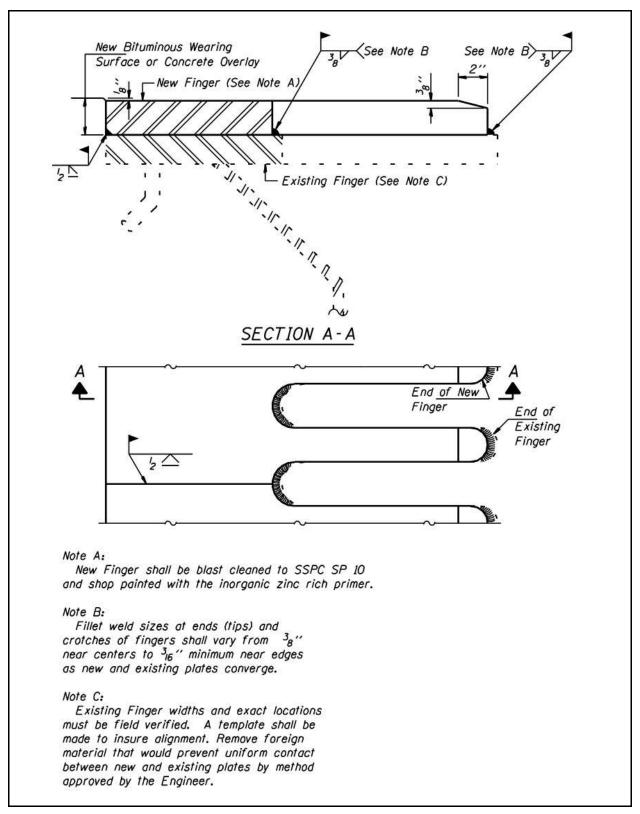
Figure 2.5-20 – Expansion Joint Treatment with Grade Raise and Existing Finger Plates
