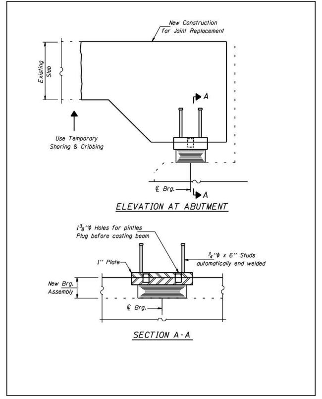
Figure 2.9-5 – Bearing Replacement for R.C. Slabs with Joint Replacement
