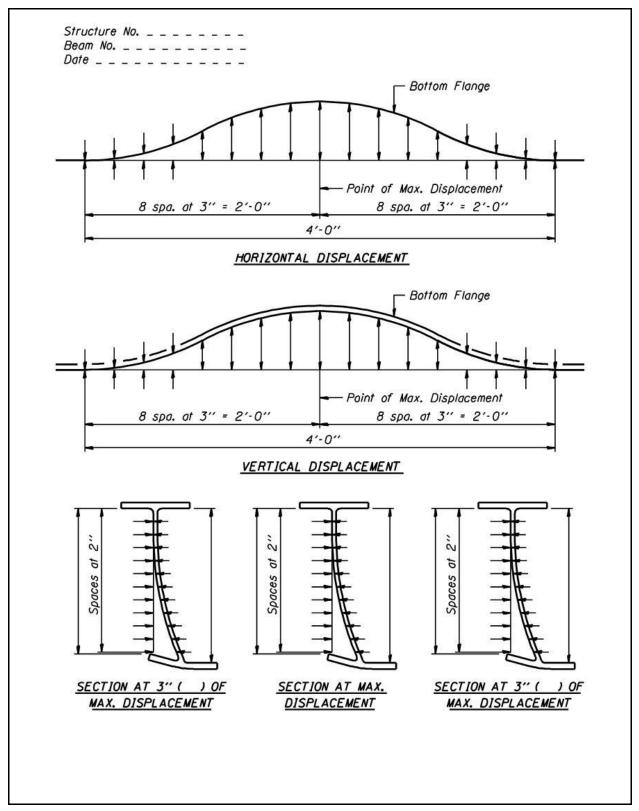
Figure 2.3-3 – Impact Damage Steel Beams
