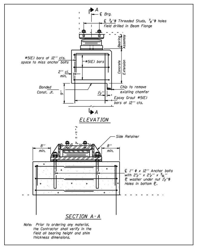
Figure 2.9-4 – Concrete Extension
