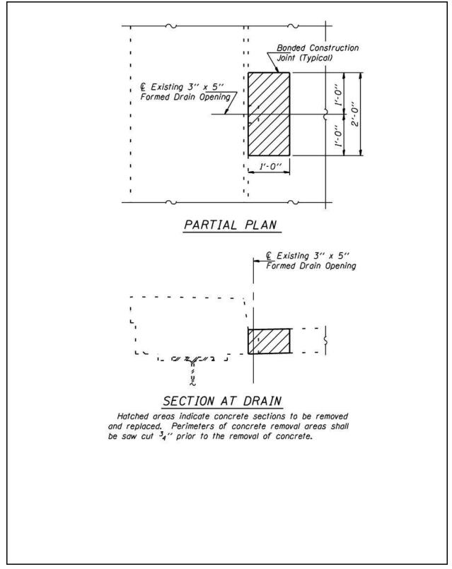
Figure 2.8-6 – Drain Elimination Detail
