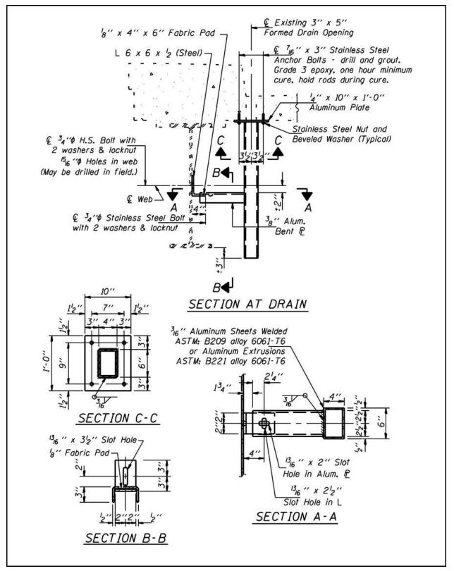
Figure 2.8-3 – Drain Extension Detail
