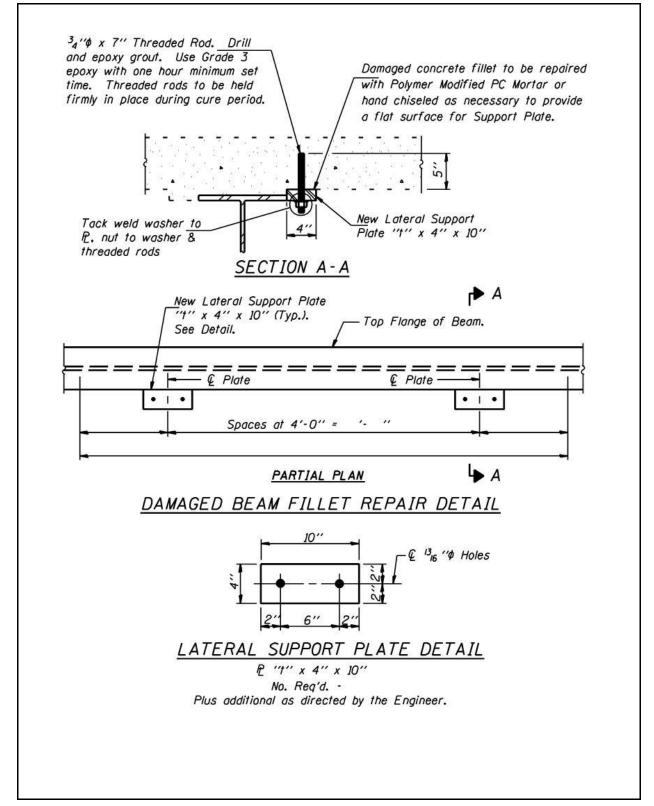
Figure 2.13-14 – Fillet Repairs and Layout of Locations
