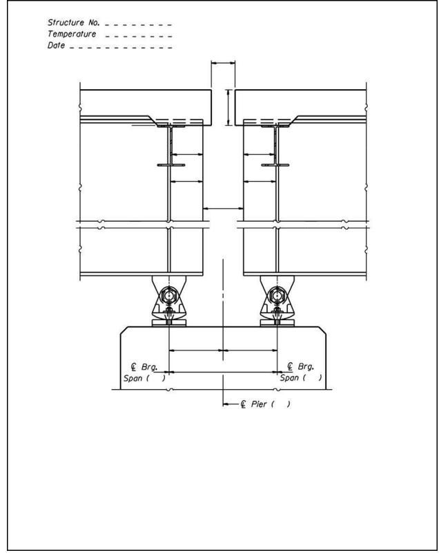
Figure 2.5-19 – Finger Joint Field Dimensions (At Pier)
