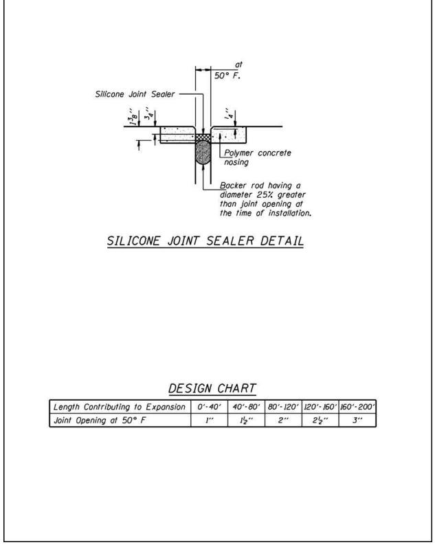
Figure 2.5-2 – Silicone Joint Sealer with Polymer Concrete Nosing
