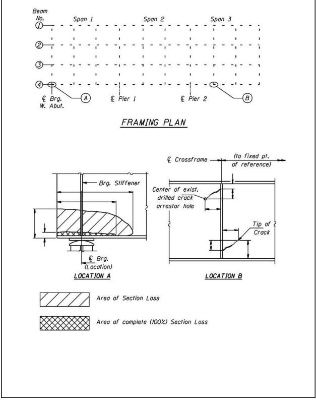
Figure 2.3-1 – Documentation of Structural Steel Deterioration
