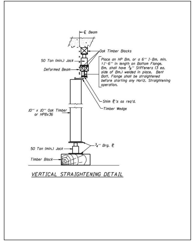
Figure 2.13-5 – Suggested Beam Straightening Methods
