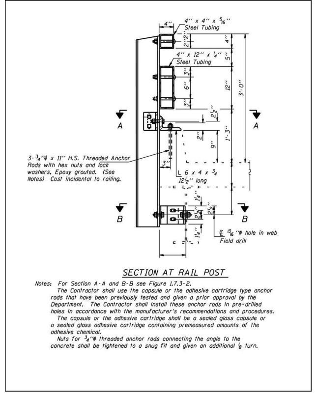
Figure 2.7-3 – Truss Rail Replacement
