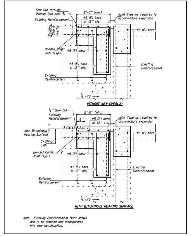
Figure 2.5-9 – R.C. Deck Girder Joint Reconstruction (Full Removal)
