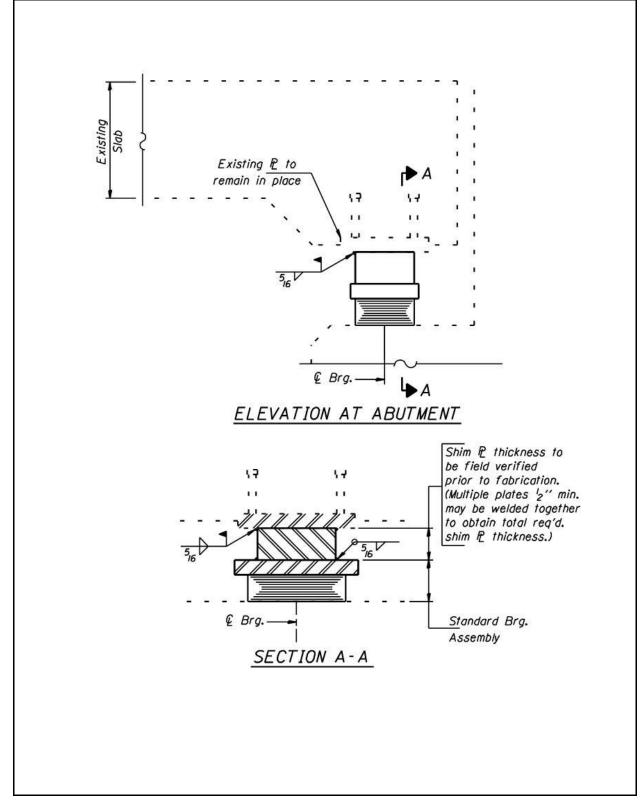
Figure 2.9-6 – Bearing Replacement for Existing R.C. Slabs
