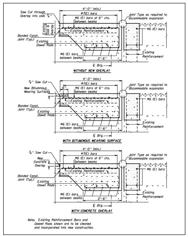
Figure 2.5-7 – Joint Reconstruction for PPC I Beams
