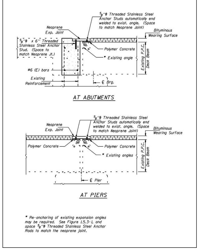
Figure 2.5-16 – PPC Deck Beam Joint Reconstruction (Neoprene)
