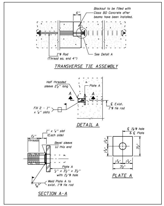
Figure 2.16-2 – Modified Tie Coupler for Transverse Tie Assembly
