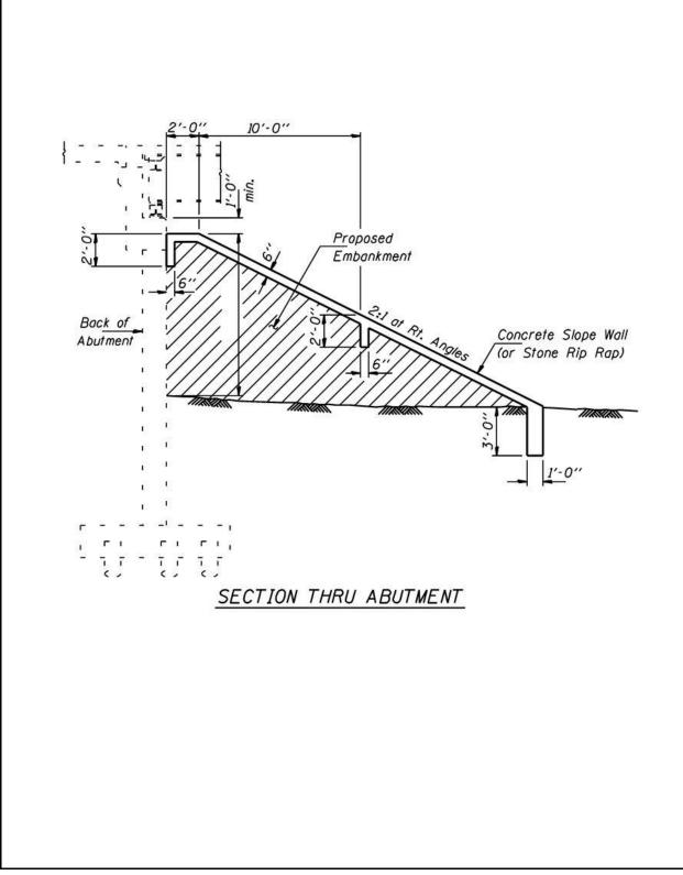
Figure 2.17-8 – Abutment Wall Support Using Embankment
