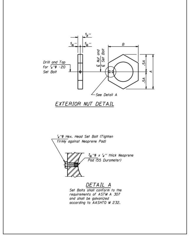
Figure 2.11-3 – Set Bolt for Pin and Links
