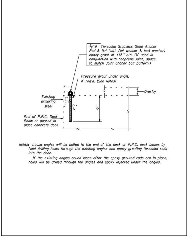
Figure 2.5-3 – Re-Anchoring Existing Loose Expansion Angles
