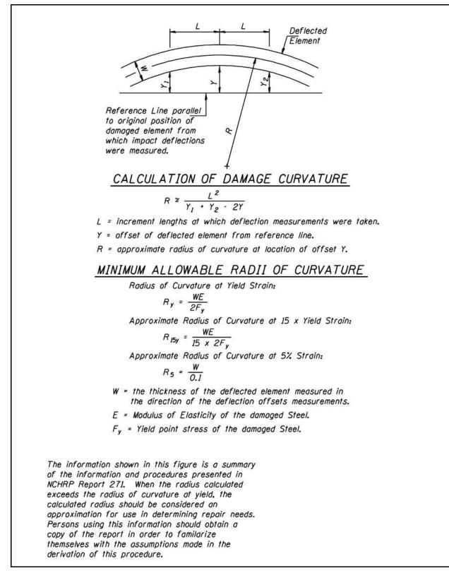
Figure 2.13-1 – Damage Calculations Based on NCHRP 271
