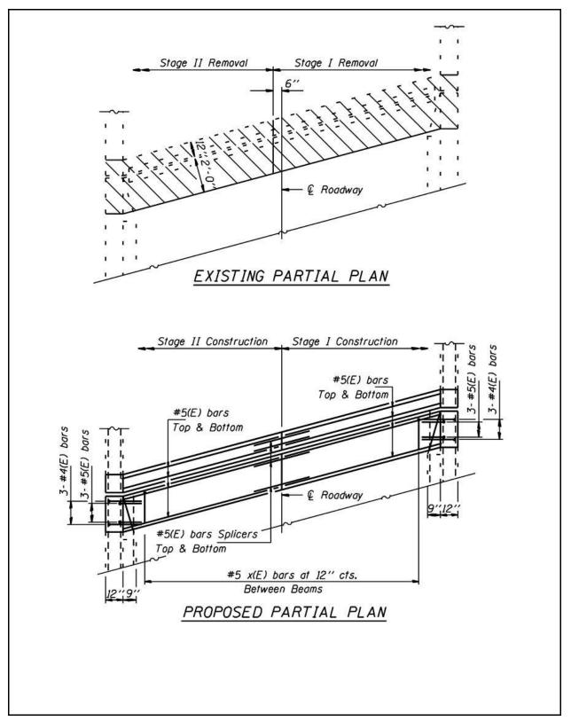
Figure 2.5-17 – Plan of Reconstruction
