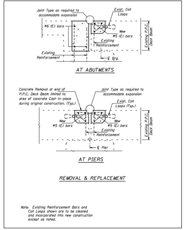
Figure 2.5-13 – PPC Deck Beam Joint Reconstruction (Blockout Removal)
