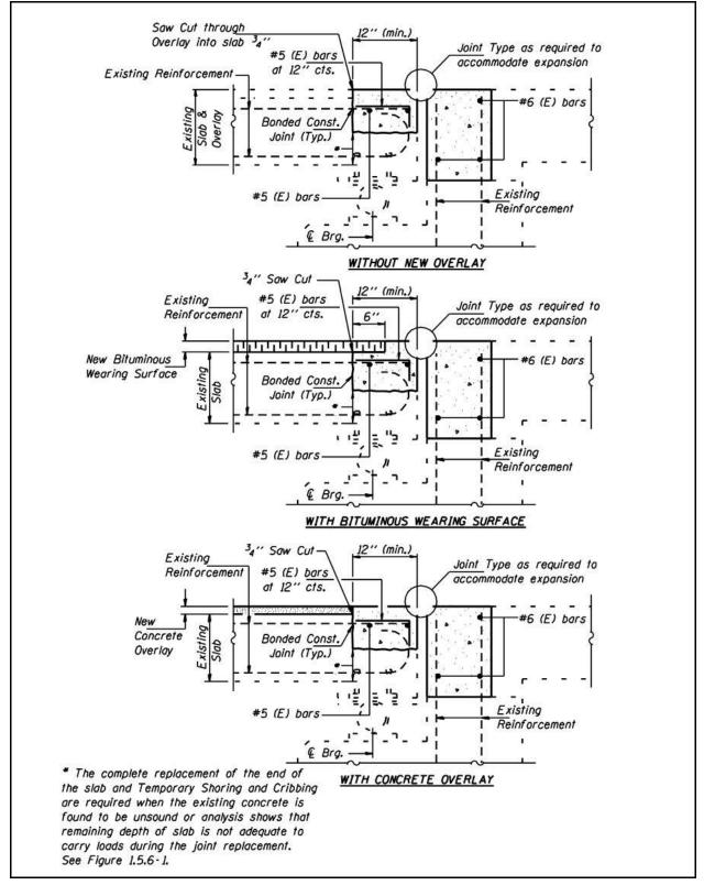
Figure 2.5-12 – Joint Reconstruction for R.C. Slab (Partial Removal)
