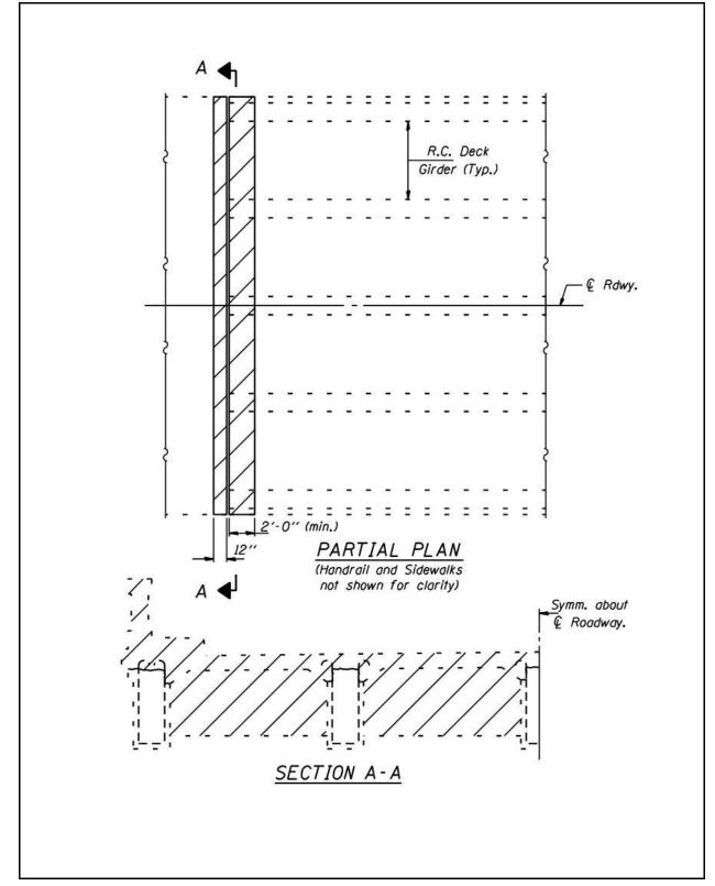
Figure 2.5-8 – R.C. Deck Girder Concrete Removal
