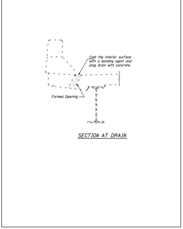
Figure 2.8-7 – Drain Elimination Detail
