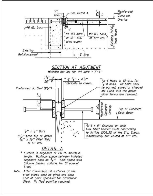
Figure 2.5-15 – PPC Deck Beam Expansion Joint Reconstruction with R.C. Overlay
