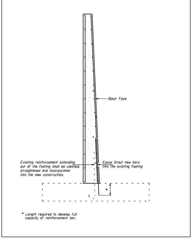
Figure 2.17-4 – Retaining Wall Stem Removal and Replacement
