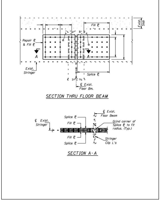
Figure 2.12-2 – End of Stringer Repair Detail
