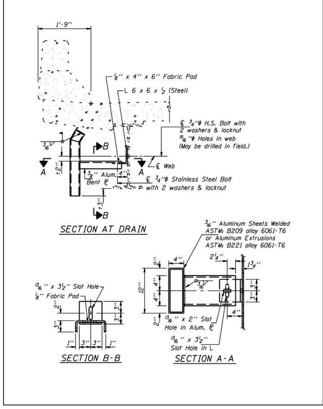
Figure 2.8-2 – Drain Extension Detail
