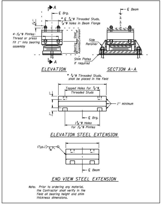
Figure 2.9-2 – Stacked Plate Steel Extension
