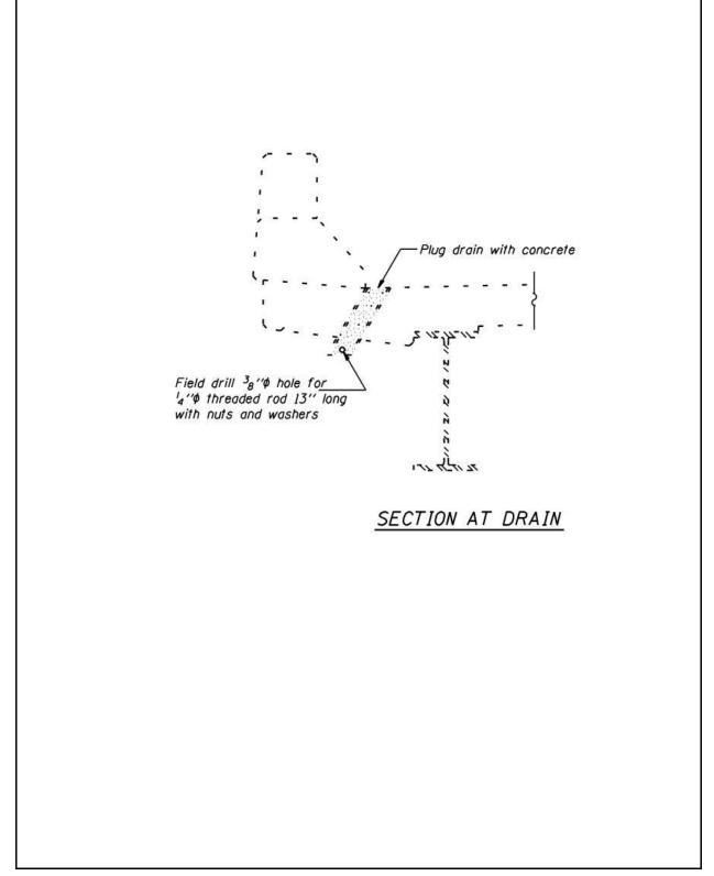
Figure 2.8-5 – Drain Elimination Detail
