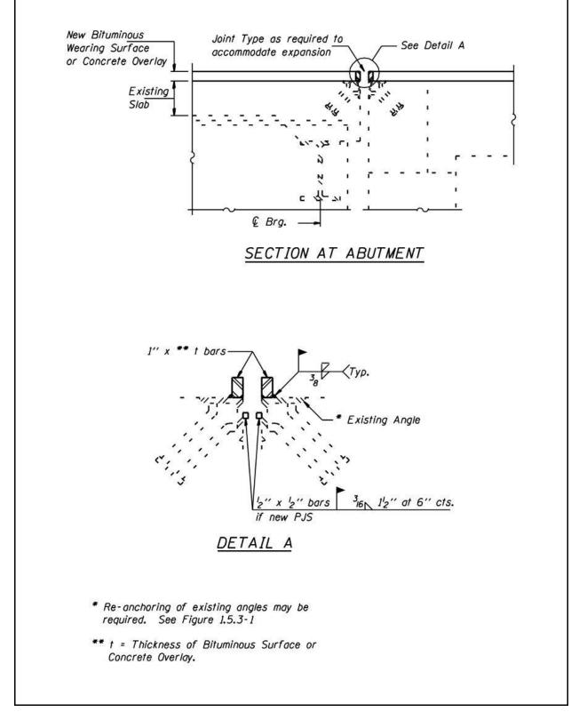
Figure 2.5-4 – Expansion Joint Treatment with Grade Raise and Existing Angles
