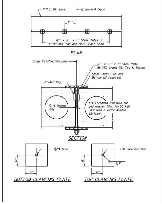
Figure 2.16-1 – Shear Key Clamping Device for PPC Deck Beams
