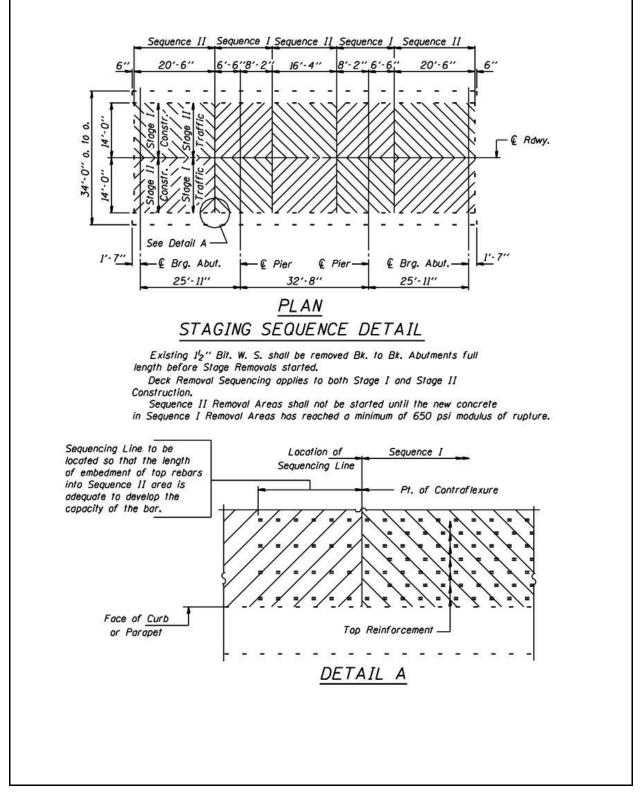
Figure 2.4-1 – Sequential Scarification and Overlaying of a R.C. Slab Bridge
