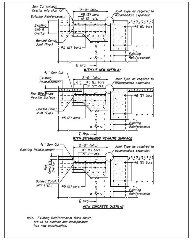
Figure 2.5-6 – Joint Reconstruction for Steel Beams
