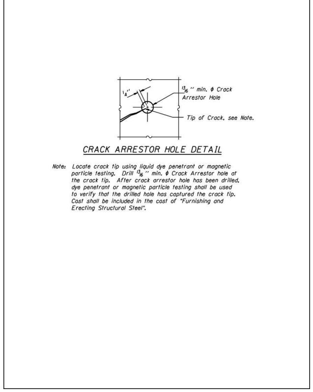
Figure 2.12-1 – Crack Arrestor Hole
