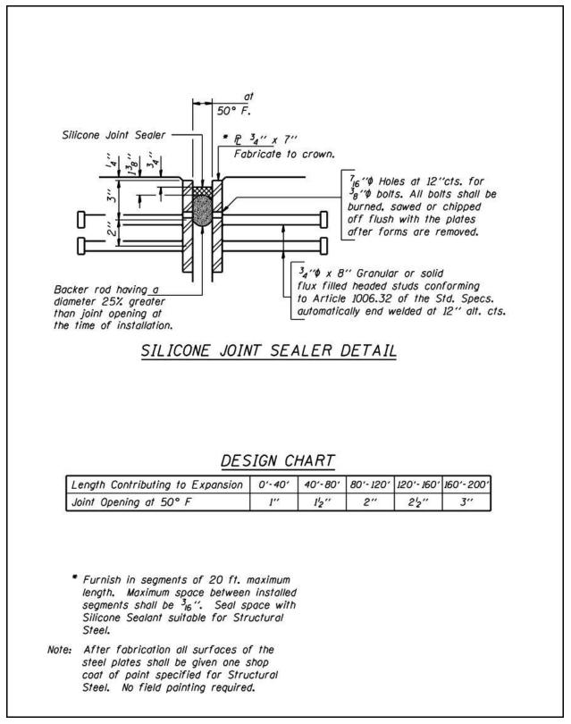
Figure 2.5-1 – Silicone Joint Sealer with Steel Plates
