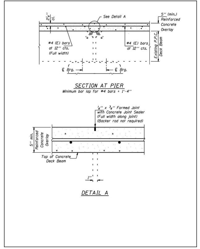
Figure 2.4-4 – PPC Deck Beam Fixed Joint Reconstruction with Concrete Overlay
