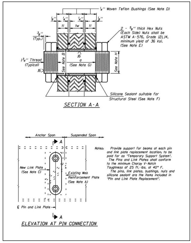
Figure 2.11-2 – Pin Replacement Detail
