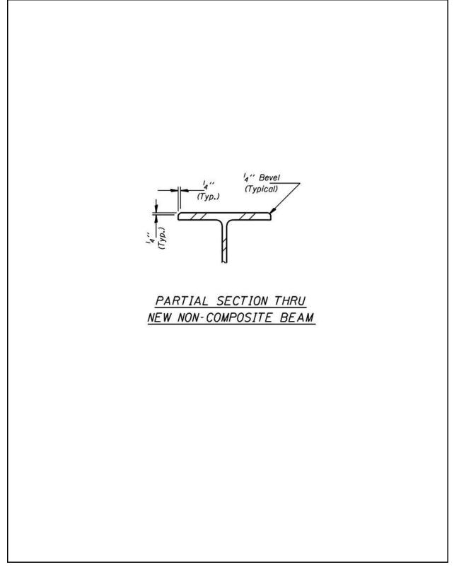
Figure 2.13-11 – Top Flange Bevel Grind Detail
