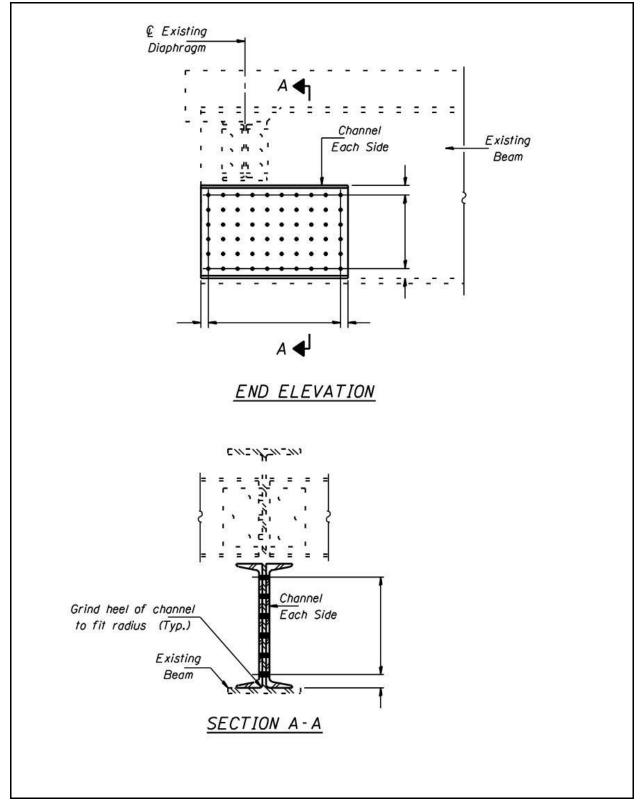
Figure 2.15-4 – End of Beam Repair Detail
