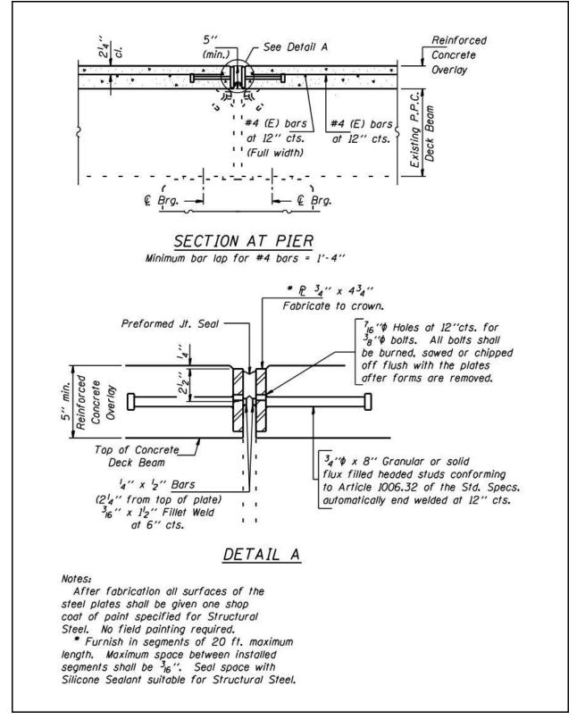
Figure 2.4-3 – PPC Deck Beam Expansion Joint Reconstruction with Concrete Overlay
