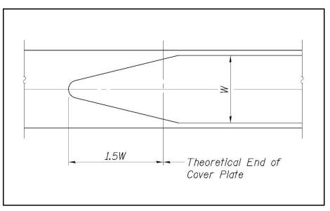
Figure 4.3-1 – Theoretical End of Cover Plate
