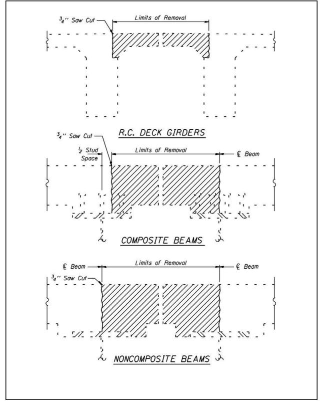
Figure 2.6-1 – Longitudinal Joint Removal Limits
