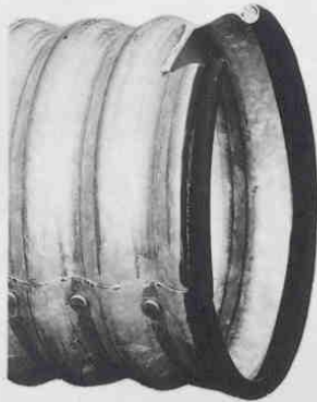
Figure 12 - Single Roll Over Round Iron Rod Satisfactory
