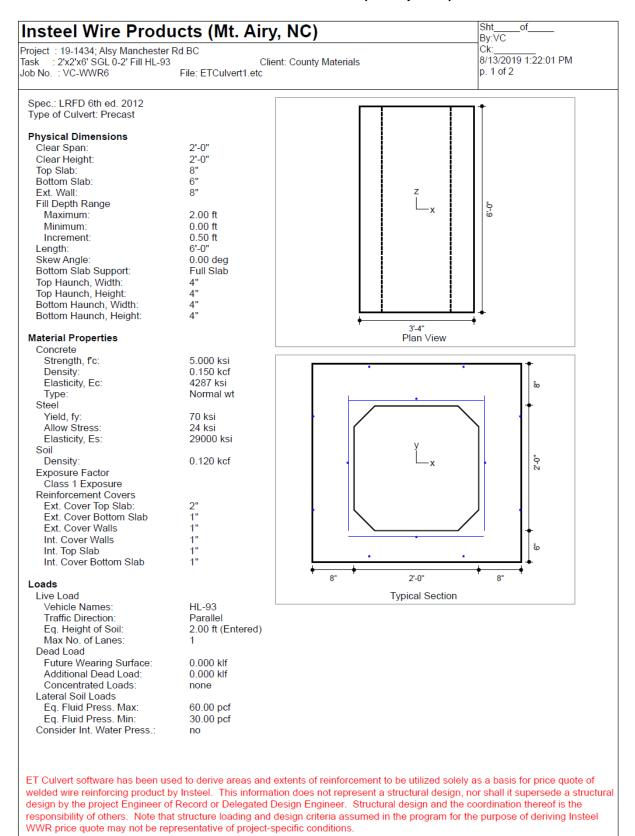
ETCulvert - Analysis and design of culverts, version 3.73
