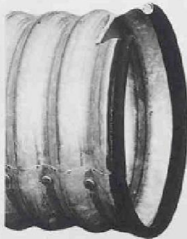
Figure 12 - Single Roll Over Round Iron Rod Satisfactory
