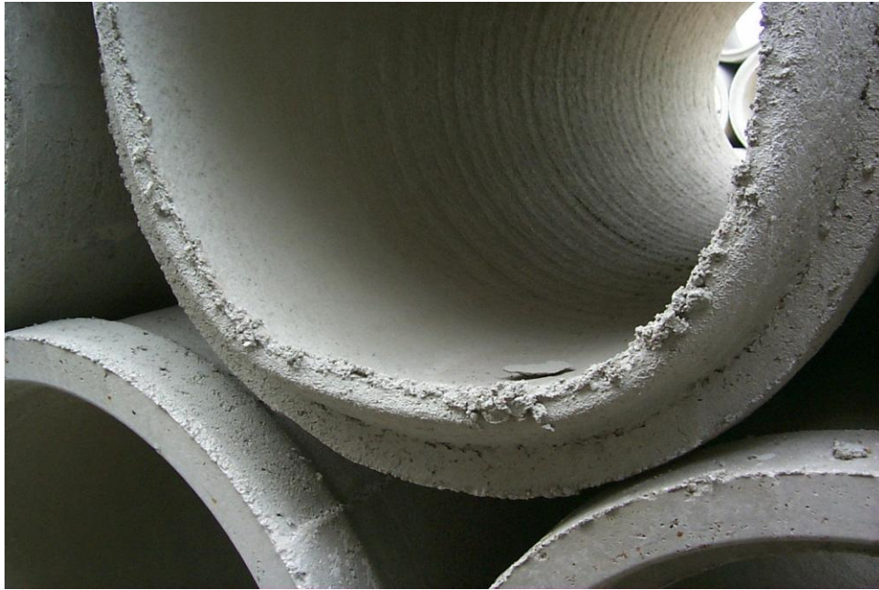
Figure 17 - Pipe Spigot Out of Round – Reject
