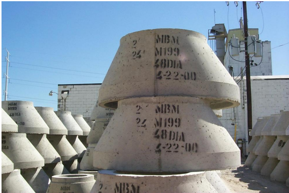
Figure 25 - Properly Marked Precast
