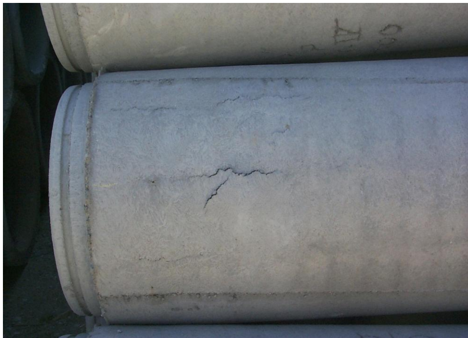
Figure 4 - Crack – Cause for rejection
