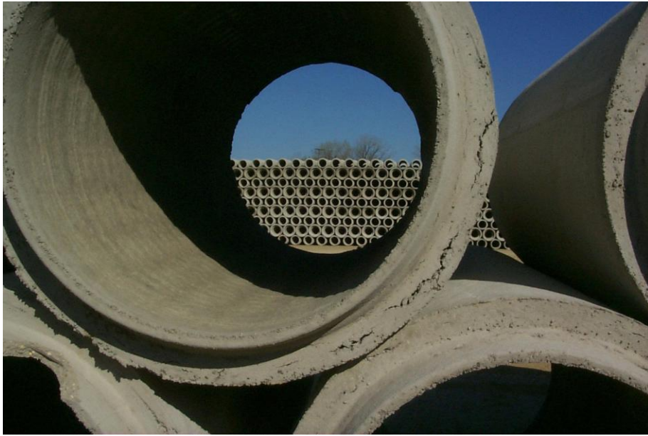
Figure 23 - Defect in Workmanship – Cause for rejection
