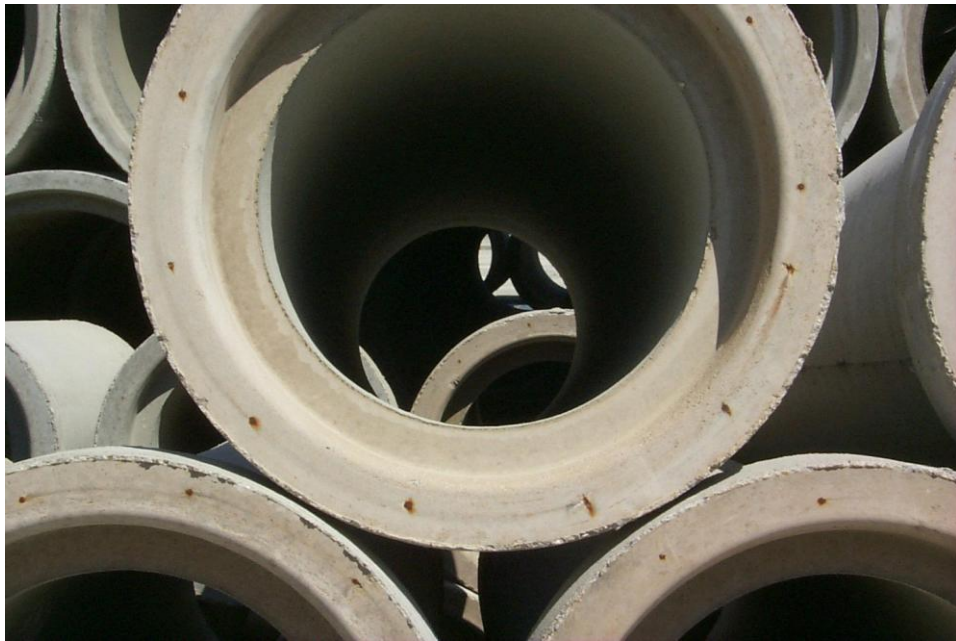
Figure 22 - Exposed Wire Ends – Not cause for rejection
