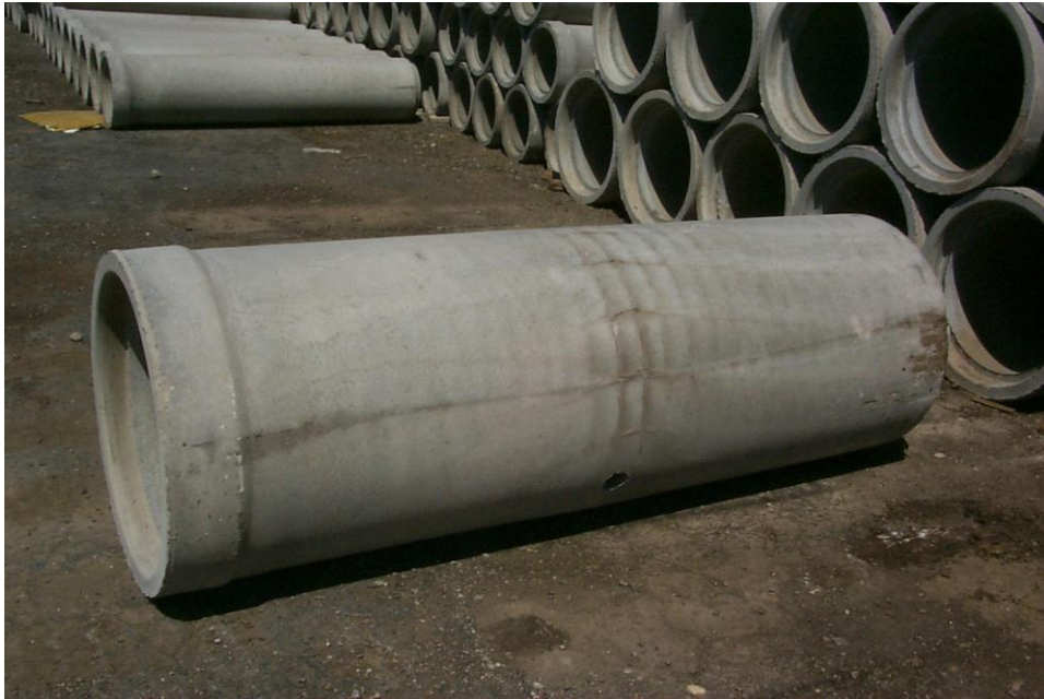
Figure 21 - Exposed Wire – Sufficient to reject
