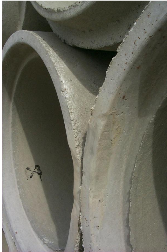
Figure 13 - Acceptable Patch in Bell
