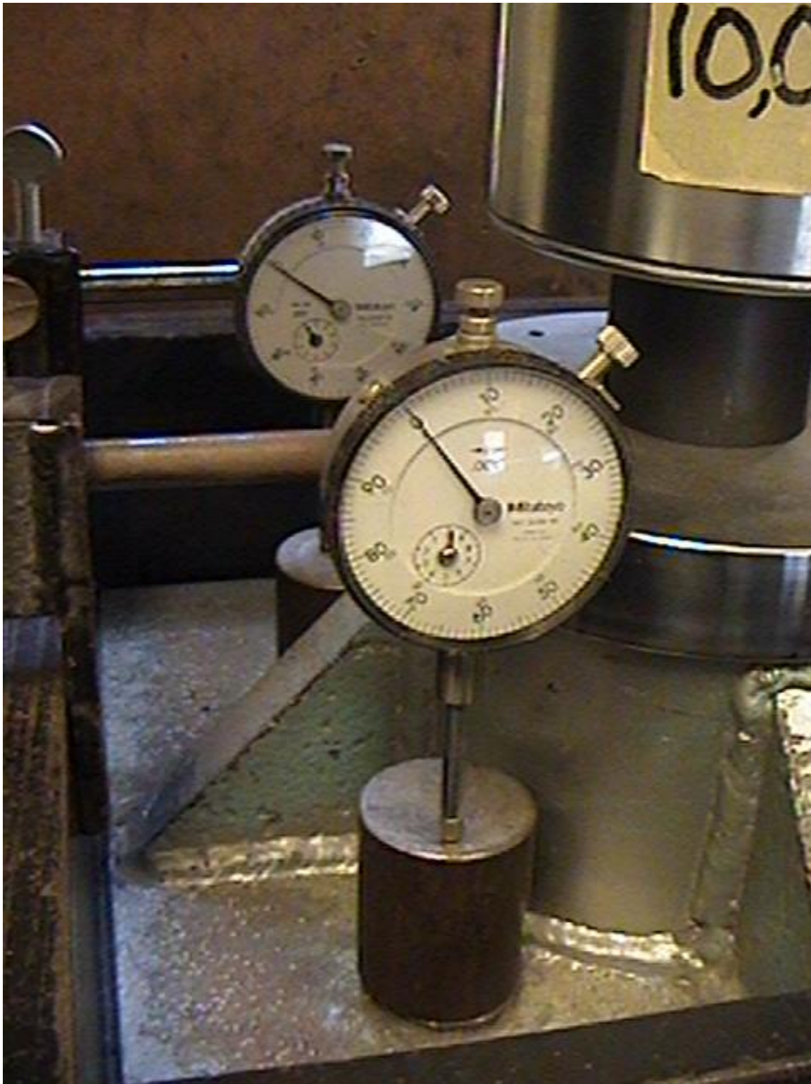
FIGURE 7. Initial preload is applied and the gauges are adjusted to zero.
