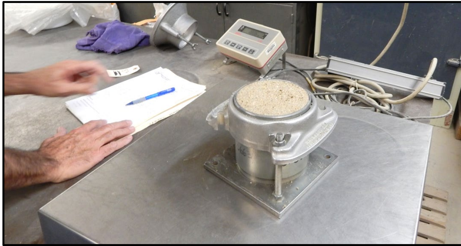
Figure 4. Photo of weighing and recording the weight of the wet soil in mold for the Proctor test.
