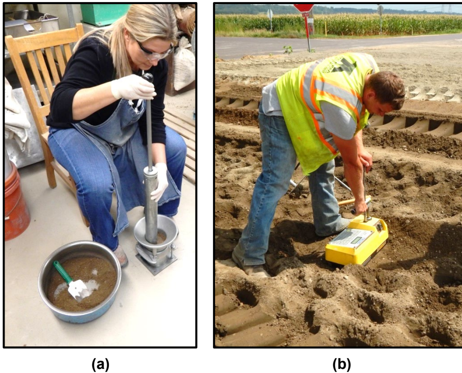
Figure 8. Photos of in-place field testing (b) of compacted dry density and moisture content tests results are compared to the Laboratory Proctor (a) test results (SDD and OMC) to determine the percent compaction and percent of optimum moisture.
