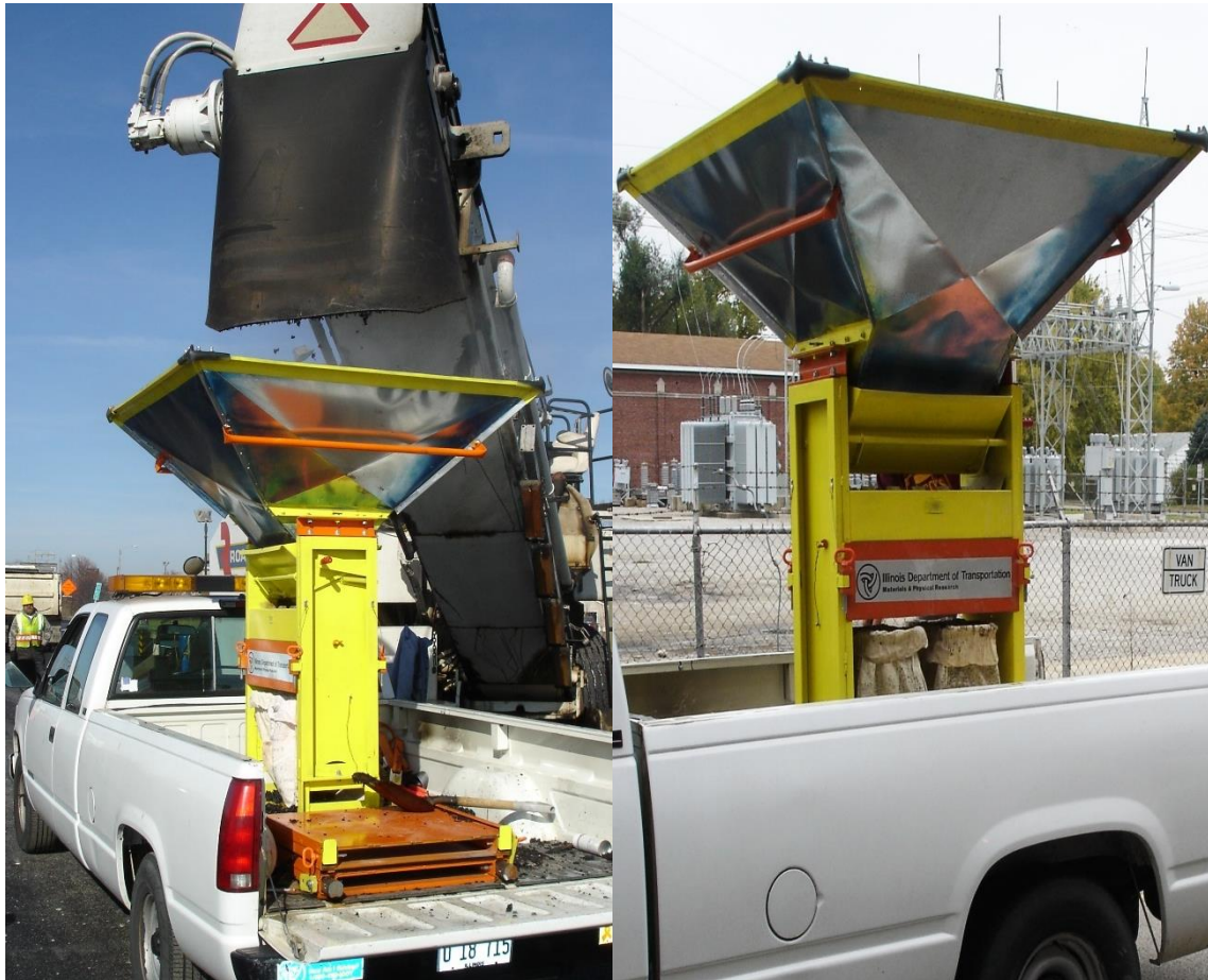
Figure 5. Additional Examples of MTD Sampling Devices
