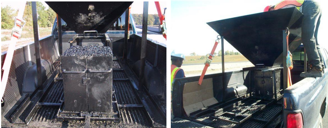
Figure 4. Additional Examples of MTD Sampling Devices
