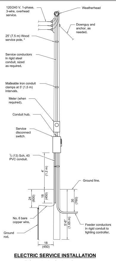
(Typical overhead service shown. Cut pole off for underground service and treat cut surface with preservative. Consult utility company standards for exact requirements.)
