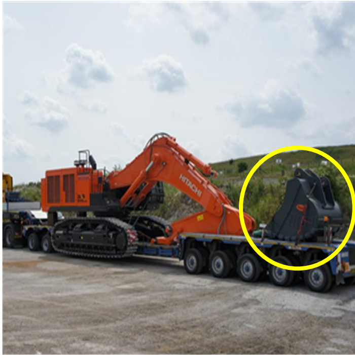
ATTACHMENTS NOT SECURELY MOUNTED ON OBJECT MOVED
