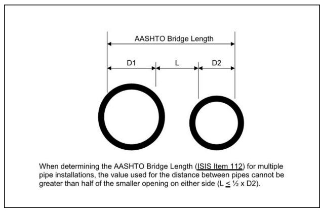
Figure 3.12-1 – AASHTO Bridge Length – Item 112 | B.G.01 for Multi-Pipe Culverts
