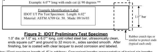
Notes: \*Test specimen length of 6" is arbitrary. Convenient lengths representative of typical pin lengths may be used. Even inch increments (7", 8", 9", 10") are recommended for ease of calibration.
