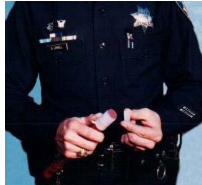
Figure 11: Remove the cap to expose the strike plate.
